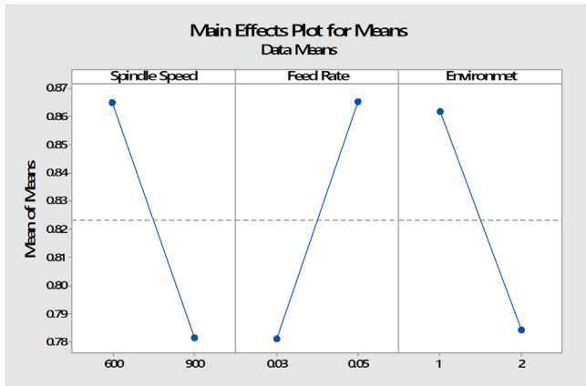
Fig. 3. Shown Main effect Plot for Means of Surface roughness (Ra).
