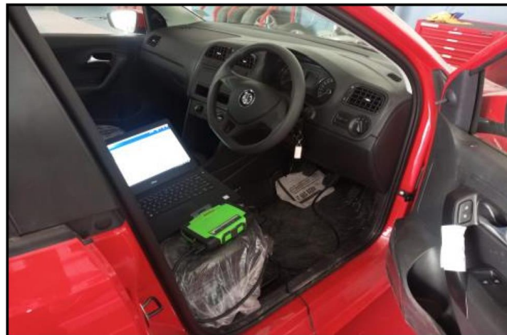
Fig. 3.2. Setup showing connection of BOSCH KTS 590 with vehicle OBD
