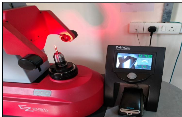
Fig. 4.10: Tool pre-setting device
