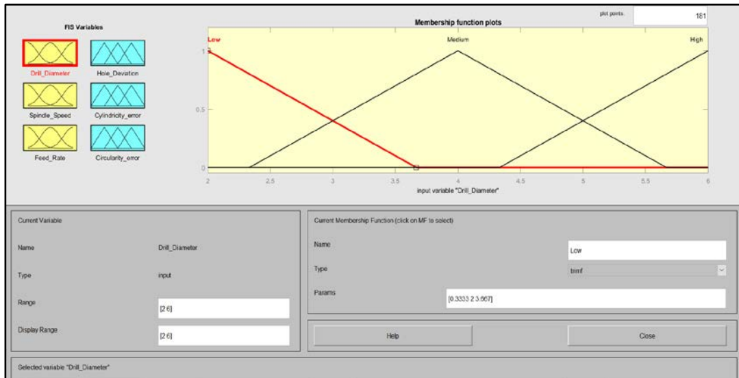
Fig. 5.48: Membership function for drill diameter
